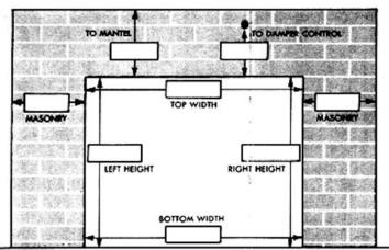
Please print exact measurement in rectangle between arrows. Measurements should be taken with steel tape and should be accurate within 1/16 inch. We make all allowances for overlap and clearance of hearth unless othewise specified.
